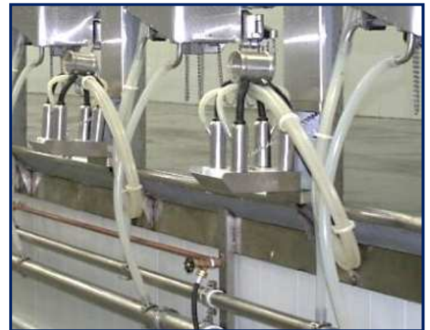
Germania's Top Outlet Claw hangs well balanced on the arm for milking and equally so in the rest position.
