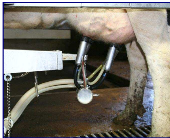
Germania's Top Outlet Claw hangs well balanced on the arm for milking and equally so in the rest position.
