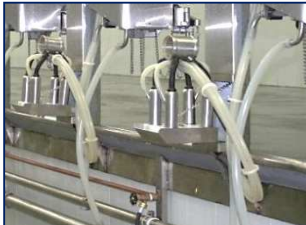
Germania's Top Outlet Claw hangs well balanced on the arm for milking and equally so in the rest position.
