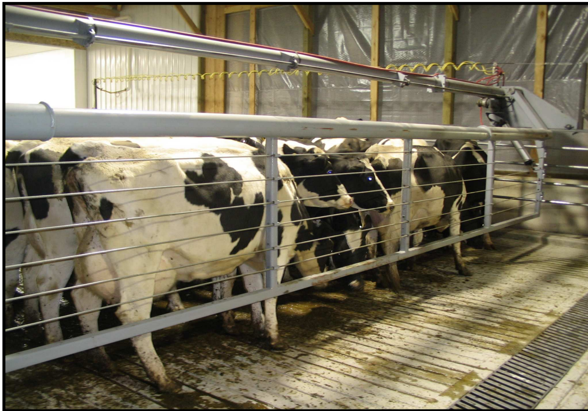
Heavy Duty, Germania Crowd Gate; Air-Powered Gear Motor - no electric controls what-so-ever. Lifts anywhere in Holding Pen and returns overhead cows to rear of pen. Air Motor shuts off automatically, both in front and back. Center-mounted Drive Unit
