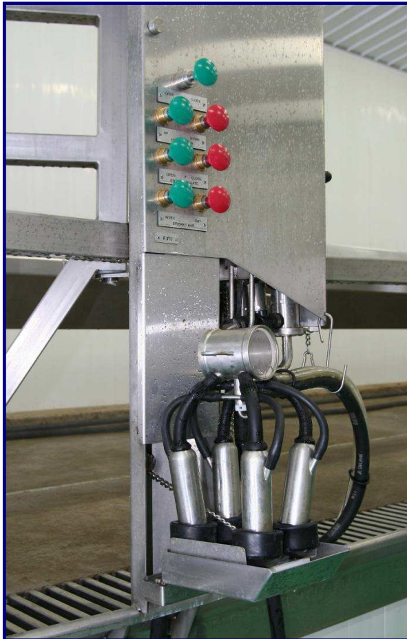
Automated Jetter Cup Holders ...open for wash-up
