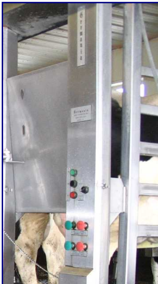
Cow Traffic Controls at last stalls on either side of parlor. Plus (2) remote panels in front. 5-Button Crowd Gate controls on one side only. Stainless cylinders operate all Gates & Automatic Indexing
