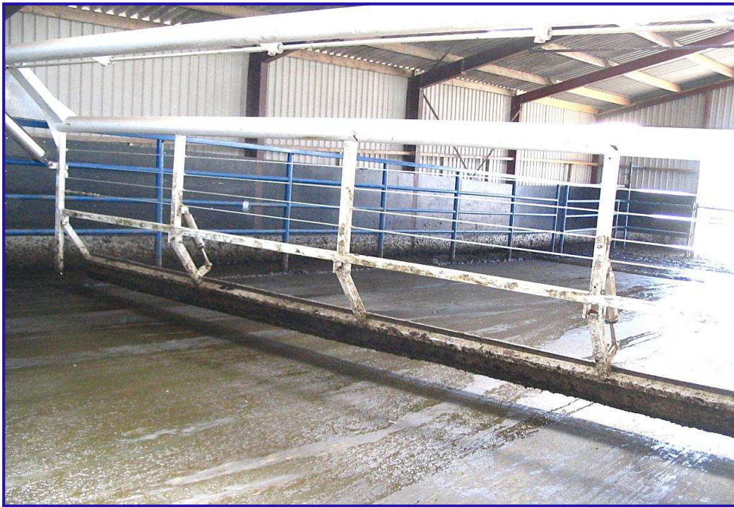
Heavy Duty, Germania-Style Crowd Gate; Air-Powered Gear Motor - no electric controls what-so-ever. Lifts anywhere in Holding Pen
