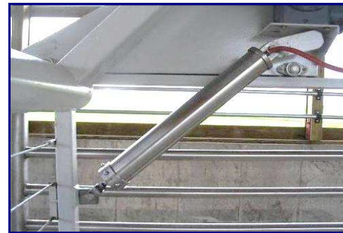
Heavy Duty, Germania-Style Crowd Gate; Air-Powered Gear Motor - no electric controls what-so-ever. Lifts anywhere in Holding Pen
