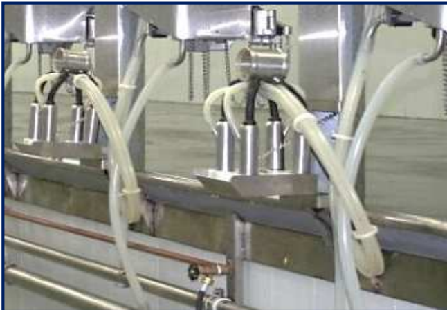
Germania's Top Outlet Claw hangs well balanced on the arm for milking and equally so in the rest position.
