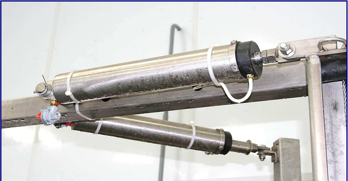
Cow Traffic Controls at last stalls on either side of parlor. Plus (2) remote panels in front. 5-Button Crowd Gate controls on one side only. Stainless cylinders operate all Gates & Automatic Indexing
