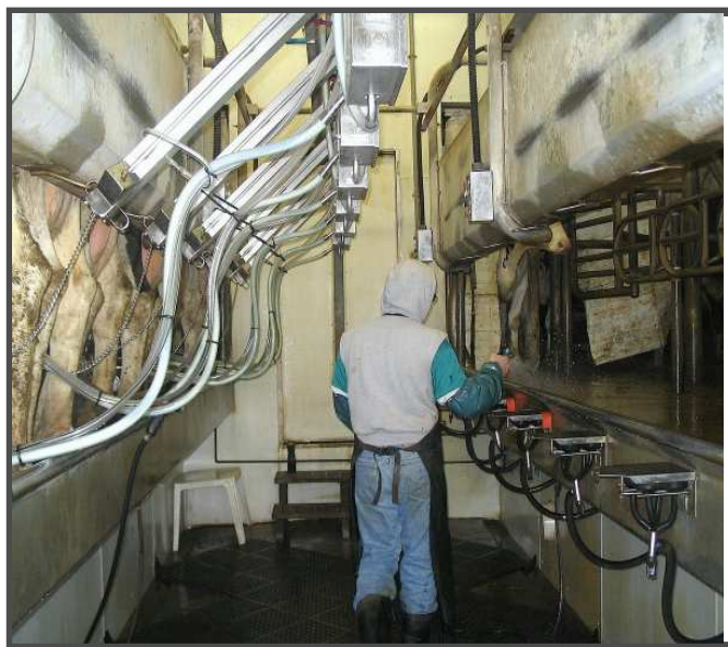
Wide open center - only the retract cylinder swings across the pit. Hoses swing with the cylinders
