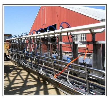
The pit wall assembly contains all below-the-curb components. We rotate the assembly up 180 dgr. for transport - as shown here
