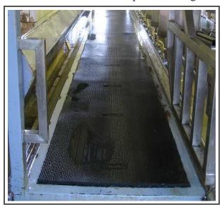
New Feature -Rubber Mats embedded into Module Base
