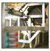
Cow Traffic Controls with(8) new Cylinders,(4) for the Gates and (4) for automatic indexing
