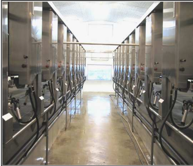
Dbl. 10 All-Stainless ProTime I HerringBone. Originally installed on a large dairy in Florida in 1989, milking 3,000 cows 3x.
