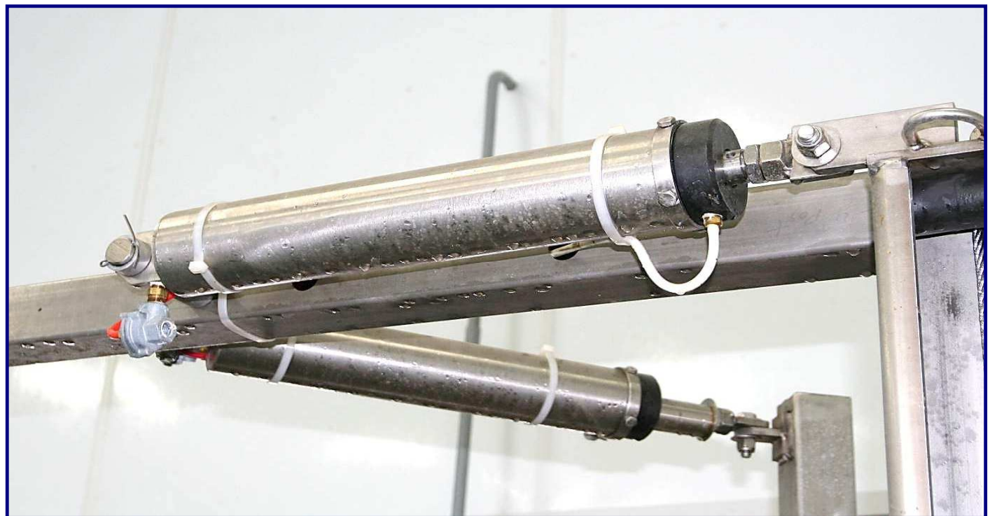
(2) Cow Traffic Controls at last stalls on either side of parlor. Plus (2) remote panels in front. 5-Button Crowd Gate controls on one side only. Stainless cylinders operate Entrance Gates & Automatic Indexing. Manual Exit Gates.
