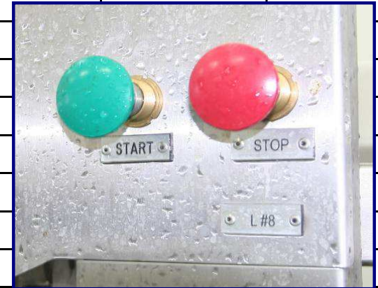
Left: Main Control station in back of parlor Center: Remote Controls in back of Holding Pen Right: Two extra buttons in front of parlor to reduce walking
