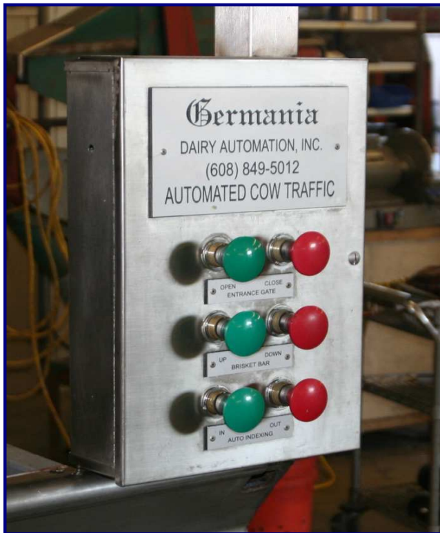
Cow Traffic Controls at last stall on either side of parlor, plus (2) remote panels in front. 3" cylinders operate Entrance & Exit Gate
